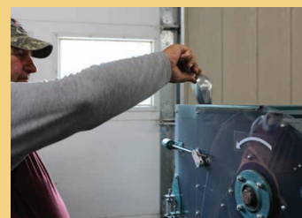
The seeds are fed into a hammer mill to break apart remaining plant material from the seeds.
